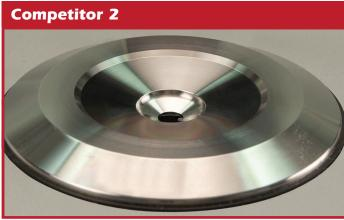
The flat open sample area has no corners to trap even sticky materials and is resistant to almost all solvents including acetone, toluene and similar organics. Choose Hastelloy option for acids like HFl and HCl.
