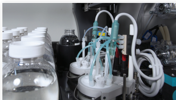
Dual titrator – higher sample throughput
