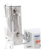
The two station dosing and filling unit is suitable for the drop-free filling of all types of different liquids.
