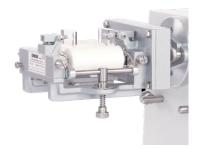
The Three Roller Mill is used for the production of ointments, pastes, creams and similar products.
