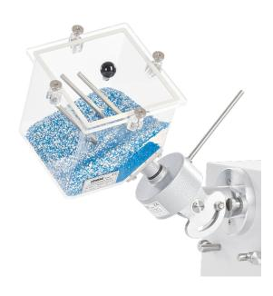
The Cube Mixer uses a tumbling motion to produce a homogenous blend within a short time. The mixing action is assisted by three stainless steel rods positioned inside the cube. The device is attached to the drive unit via the ERWEKA Universal Gear UG, which permits operation at various angles for optimal efficiency. Our cube mixers are available in the following versions:
