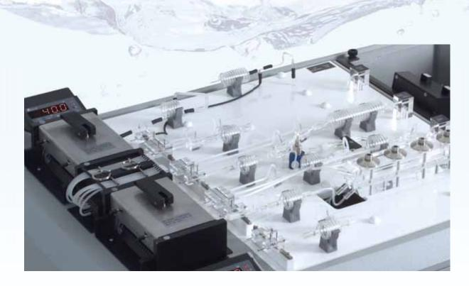
The San<sup>++</sup> chemistry section consists of a pump unit, an air segmentation injector, chemistry application modules with individual waste receptacles and data detection with digital detectors.
