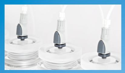
Thanks to this new cell concept, the cells can be mounted easier to the new flow-through tester DFZ II and thus enable a faster preparation and performance of dissolution tests.
