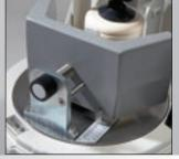
Imbalance compensation with simple mechanical adjustment
