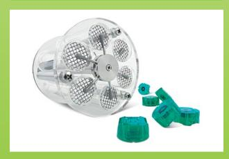
The optional mBasket for automated testing uses a magnetic guided disc and sensors under the USP/EP compliant sieves.
