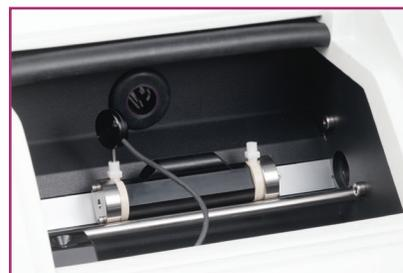
Place the TempTrol™ cell in your TempTrol™ equipped Autopol 880T sample chamber to measure within  $\pm 0.2^\circ\text{C}$  of the ICUMSA specified temperature (normally 20°C or 27.5°C). Any temperature between 18°C and 35°C may be selected.
