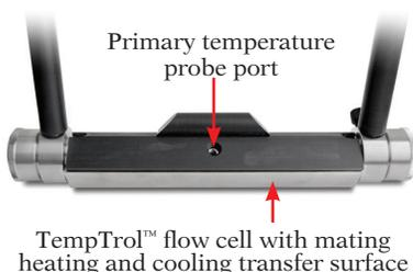
Rudolph 41T style cells allow for Electronic Temperature Control to a defined set temperature (i.e. 20°C or 27.5°C)
