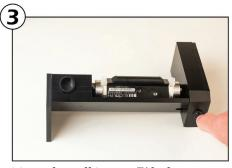
Turn the FillStation<sup>™</sup> light on. The light will turn off automatically after a few minutes.
