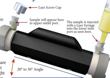
Syringe. When the sample appears near the top outlet port, simply place the Luer cap on the upper port and then lower port. Your cell is now filled, capped and air bubble free. Cells must be clean and dry to ensure proper filling with minimum sample.
