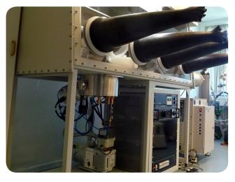
A modular MiniLab 026 system for installation into a glovebox
