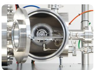
Load-lock chamber customised with a substrate gas-cooling station
