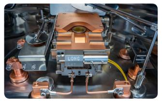
Telemark multi-pocket water-cooled electron-beam source
