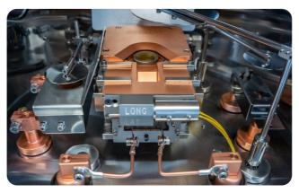
Telemark multi-pocket water-cooled electron-beam source
