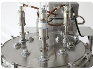
$\label{thm:minimum} \mbox{Minilab 125 chamber roof, with removable top-plate allowing for future re-configuration}$
