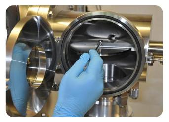
Inserting substrates into a MiniLab 125 load-lock
