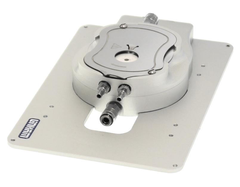
**Rotating Quartz Window**For continuous sample observation and high resolution imaging
