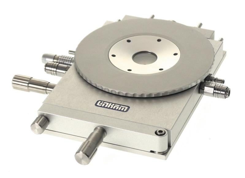
**Heating and Freezing**Temperature range from −196°C up to 600°C
