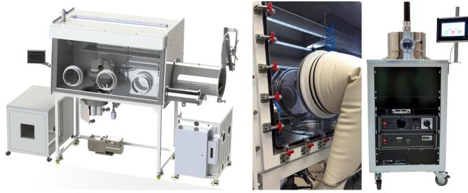
Above: Installation configurations for MiniLab 026 etch/anneal stations. Left and centre: Model and photograph of unit with etch and anneal stages interfaced with glovebox base for easy operation through gloveports. Right: MiniLab 026 tools are also available as standalone systems, where glovebox integration for sample handling in inert environments is not required.
