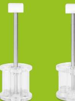
AirBasket type A (with 6 test tubes, for ZT 730 series only)
